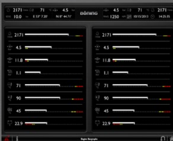
The bar graph presentation makes for easier reading of important engine parameters, thus allowing for quick visual comparisons.
