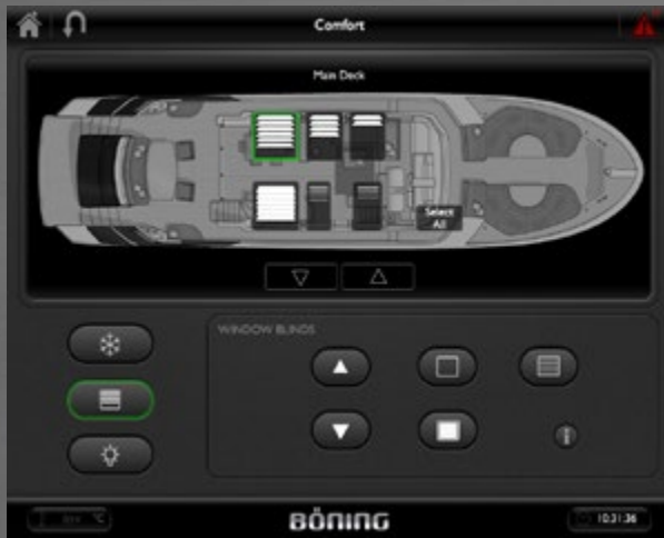
Remote control for air conditioning systems, lights, and blinds on a single page, displayed in switchable deck views.
