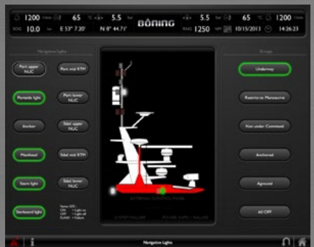
Navigation and signal lantern control and monitoring.
