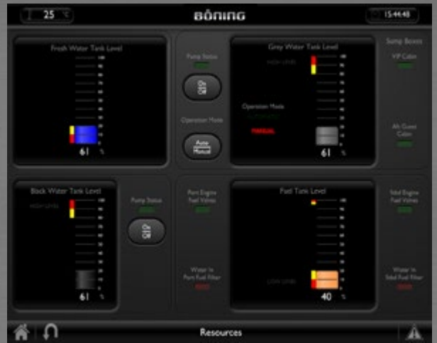
Fuel, water, oil, and other resources are carried along in tanks most of the time – as well as waste water and sewage. Bar graphs display the tanks' filling levels states. The pumps can also be controlled from this page.
