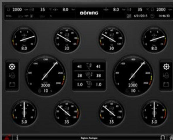
Just like in your car: The display provides information about the engine's state, using customary display systems. The engine data are displayed on round instruments and in numeric presentation.
