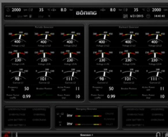
On-board power grid monitoring, including generators and battery chargers.
