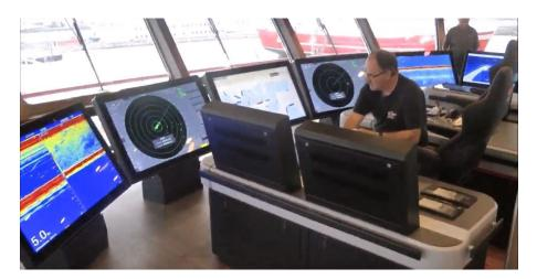
The Bridge Automation and seamless control are key functions for vessels that required efficiency and productivity. Check out an example where the Böning system was custom designed to achieve all these goals. Three 24in touch-screen Böning controllers have various presets, enabling the operator to quickly select preferred displays in relation to this boat prevailing mode of operation. This isa 82m fishing vessel, equipped with Böning Furuno Video Wall for Bridge Automation.
