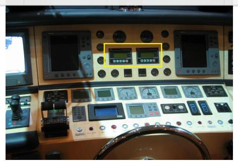
The MMDS-LC display is part of the second generation of Böning Electronics for MAN marine diesel engines. Click below to check how to upgrade to the latest technology of engine monitoring.
